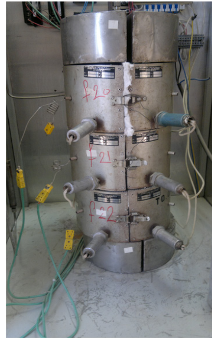
Figure 1. FTS fixed-bed reactor used for experiments
