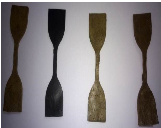
Figure 1. Cured samples from left, CIIR/NR, CIIR/NR-graphite, CIIR/NR-graphen oxide, CIIR/NR-C 15A
